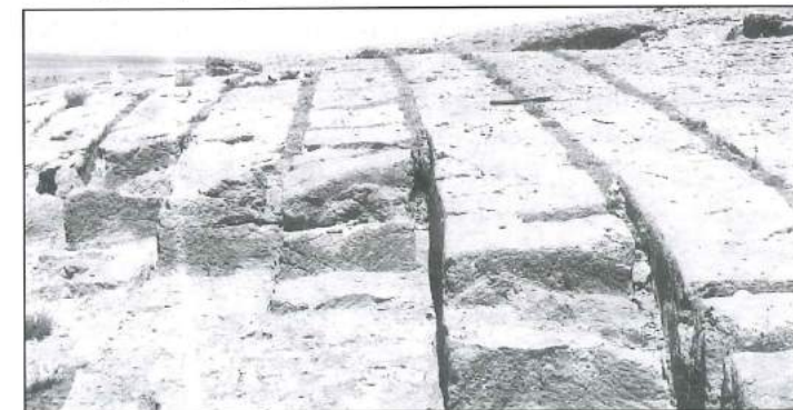
4. Al-Qaṭrāna quarry: channelling operation.
