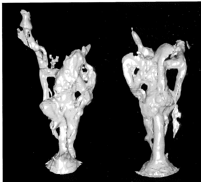
3. Three-dimensional reconstruction of the cavity inside the casting mould shown in FIG. 2 after tomographic data. Front and back view. Height of figure: ~60mm (C. Röffke).
