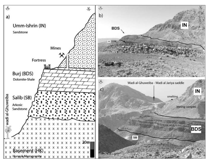
4. The geology of Rās al-Miyāh: a) a schematic section of the rock formations in the vicinity of the fortresses, looking west. Note the copper ore bearing horizon of Burj formation, the mining technique, involving shafts dug into the lower part of Umm-'Ishrīn formation and the topographic step caused by the erosion of the soft shale unit of Burj formation; b) Rās al-Miyāh *East* and the geological formations, looking west; and c) Rās al-Miyāh *West* and the geological formations, looking west.
