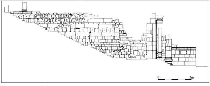
9. Elevation of north wall of Propylaeum (WB).
