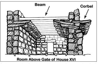
2. An example of corbel and beam roof construction from House XVI at Umm al-Jimāl (adapted from de Vries 1998: fig. 65).
