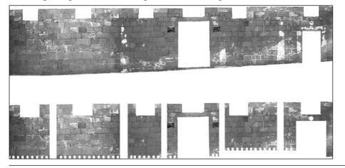
10. Hallābāt: reconstruction of the bichromatic decoration of the court walls (note the canopies with the same colour scheme). A: Traces of decorative plaster applied to the basalt-built walls of the main court in the palatine section of the complex. B: Reconstruction of the decorative pattern of the white mortar plaster; note the combination of 'pilasters' and the dado with the crown of 'heads'.
