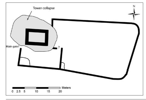
7. Wall plan of Rās al-Miyāh *West*. The width of the inner walls of the tower is approximate.
