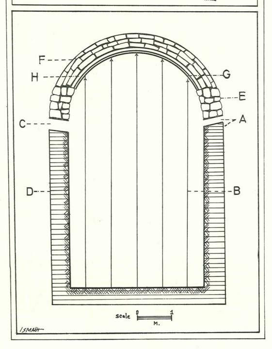
be burnt are laid in a dome without mortar so that they will not fall into the pit after the wood is burnt. This same method of dome construction can still be seen in old village houses.
