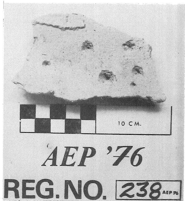
Pl. LXI, 3 - Site II, fragment, showing "pecking" techni- que for keying plaster coats.
