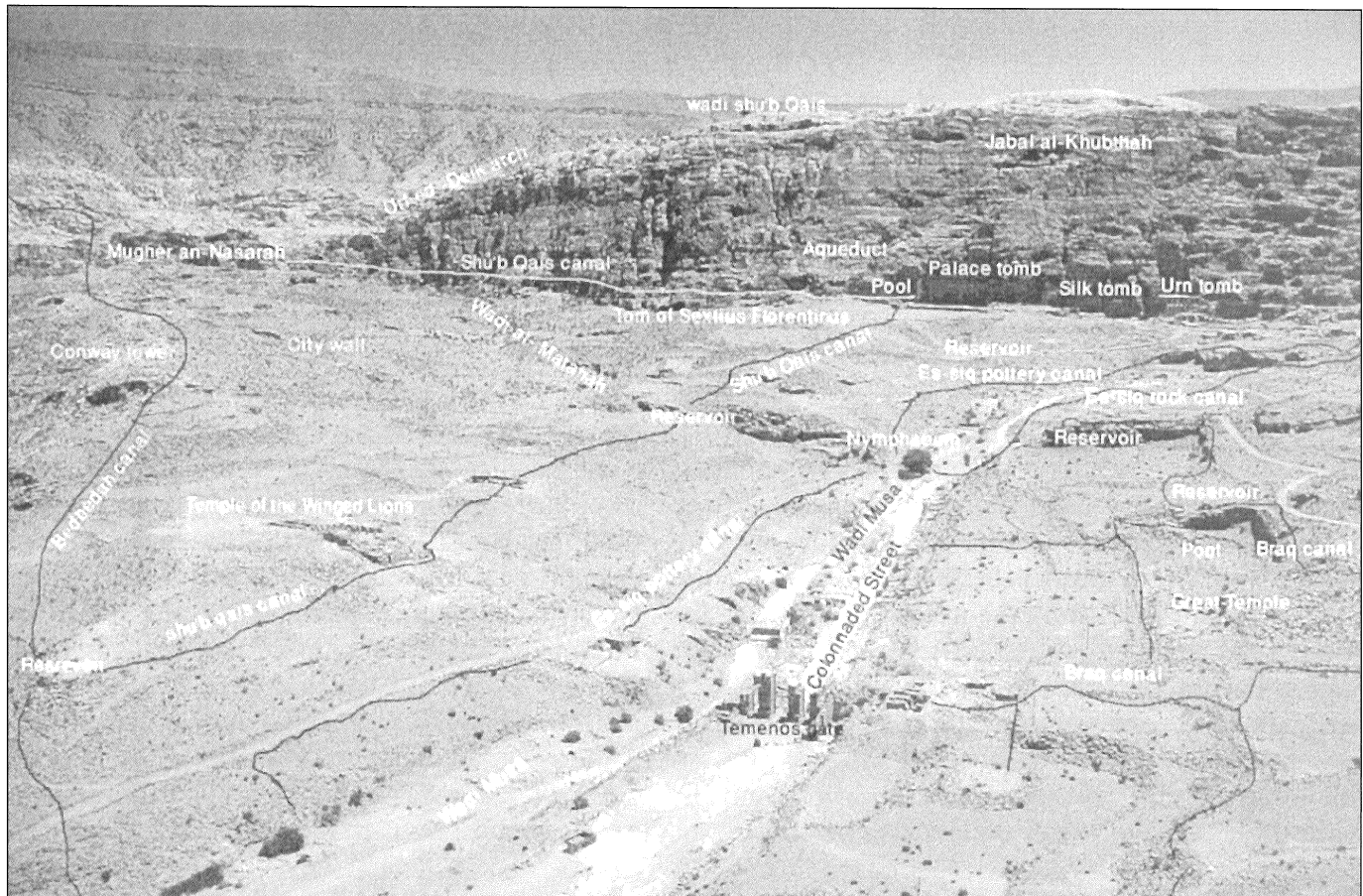
2. Aerial view of the center of Petra (1980) showing the water distribution system.
