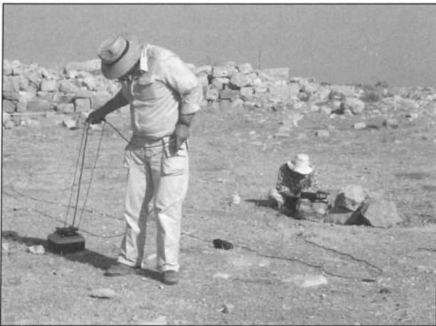
4. John Hakes and Bruce Routledge conducting the ground penetrating radar survey.
