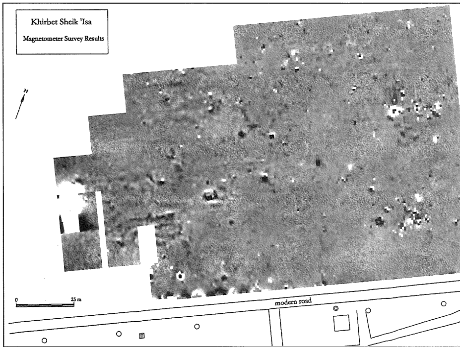
5a. Results of the magnetometer survey at KSI in the form of a grey-scale plot (Geoplot 3: shade plot (clip), black and white tones are +17 nT and -17 nT respectively).
