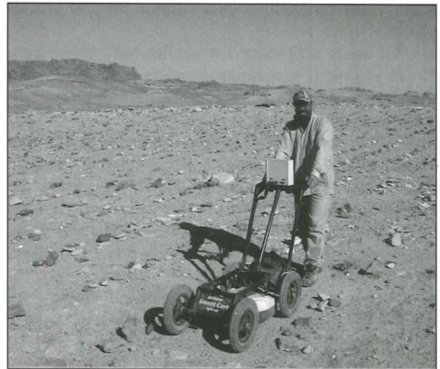
13. Mr. Jamal Saffi pushing GPR unit in cleared lanes, E116.
