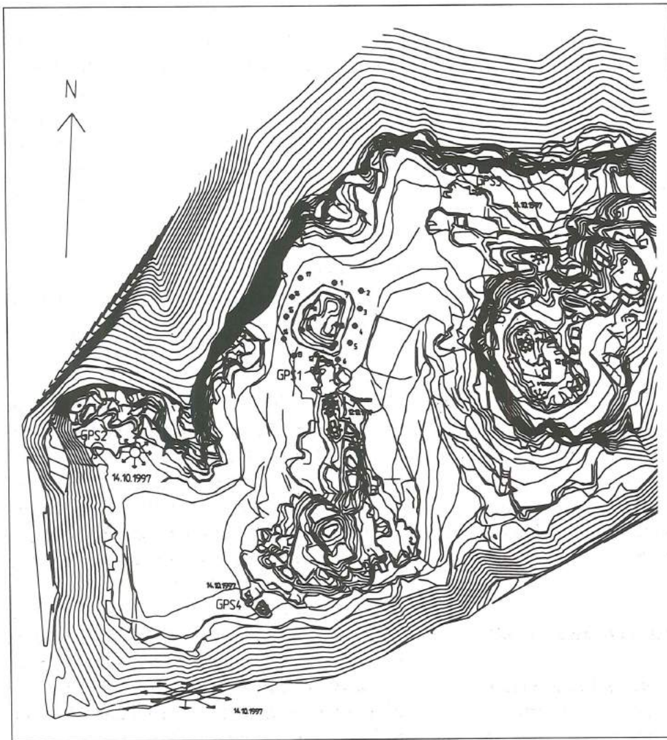
1. A topographic map of Jabal Hārūn mountain produced from aerial photographs. The map contains contours (5 m intervals), break lines and structures (created by the cartographic team under the direction of Henrik Haggren, Helsinki University of Technology).
