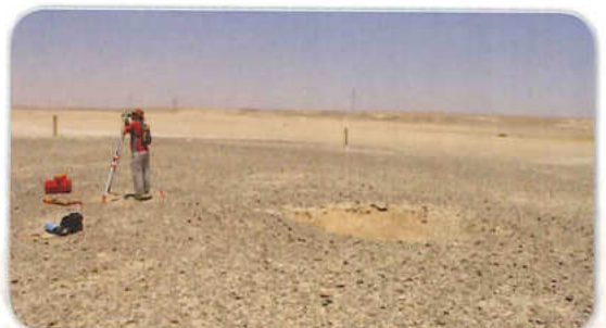
Fig. 3 : We surveyed the site to produce a topographic map of the site and relocate old excavation trenches (excavation trenches visible in the background).
