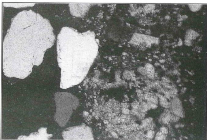
9. Last preparatory layer for painted surface, made of fragments of carbonate rocks and lime (n+, ~50x).
