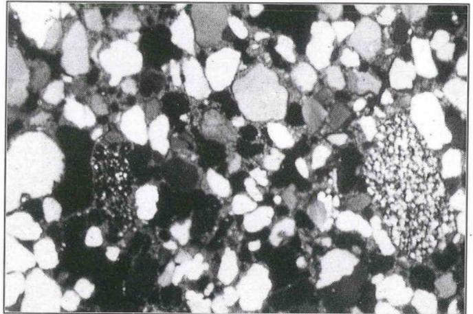
8. Sample of first layer of mortar underlying the Petra frescoes viewed under optical microscope. The granulometry is somewhat dispersed. Some siltstone is visible (n+, ~25x).
