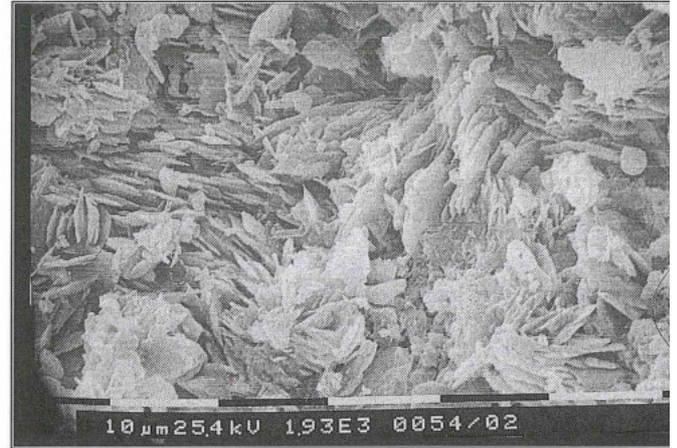
3. Closely packed microcrystals of calcium sulphate (SEM).
