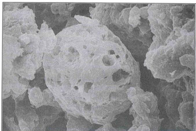
10. Carbonaceous particles on painted surfaces at Bayda (SEM).
