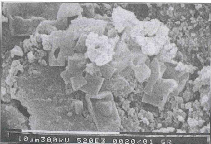
7. Partially dissolved sodium chloride crystals (SEM).
