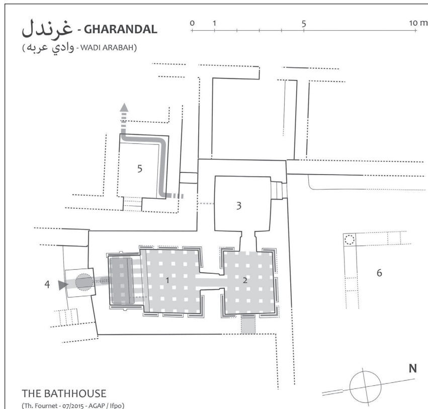
2. Plan of bath – 1. Caldarium ; 2. Tepidarium ; 3. Frigidarium ; 4. Praefurnium ; 5. Latrine; 6. Courtyard (Th. Fournet).
