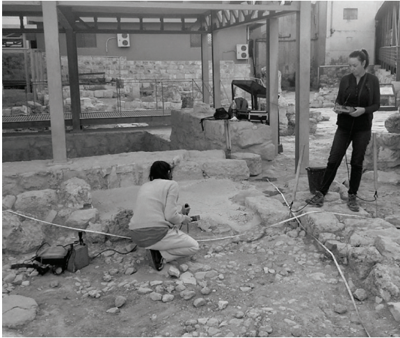
11. Georesistivimeter analysis (courtesy of MRAMP).
