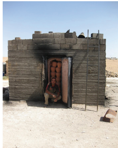
5. New kilns fueled with recycled diesel fuel for oxidation firing only.
