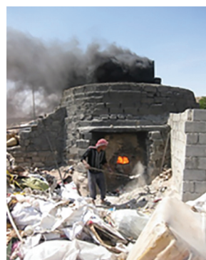
3. Round updraft kiln during a reduction firing.
