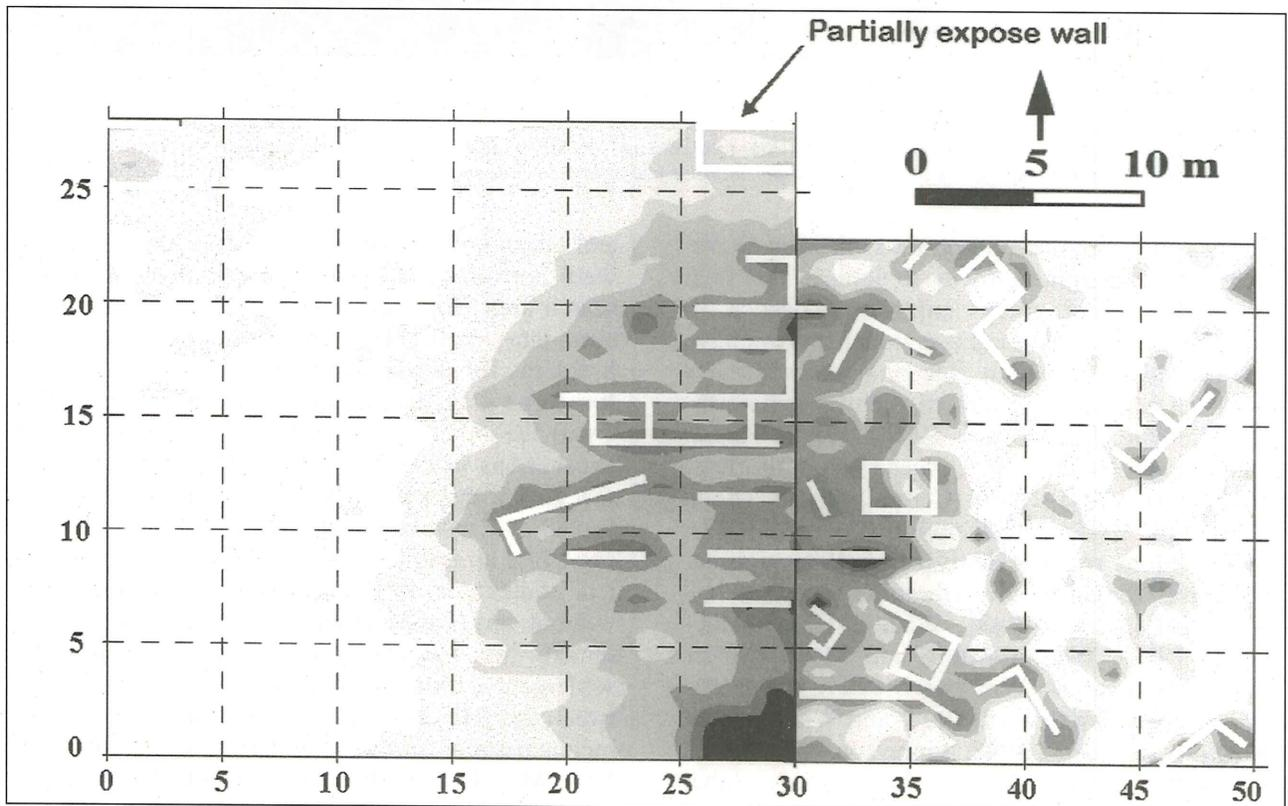
7. EMI (Electro Magnetic Induction) data acquired at the WFD 001 site rendered as gray levels. The buried stone walls appear as relative lows and are rendered in black and shades of gray. The superimposed white lines are the interpreted location of walls. All dimensions are in meters.
