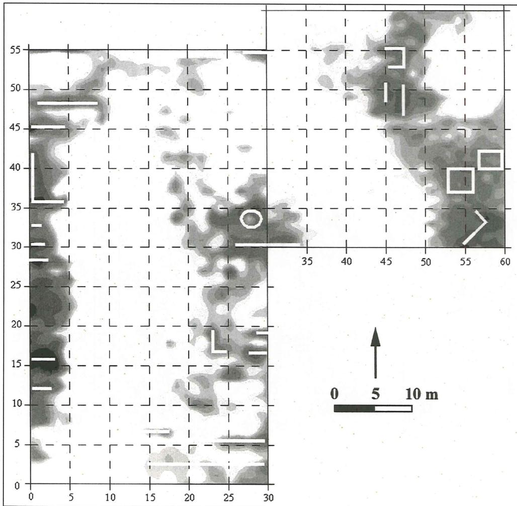
9. EMI data acquired at the Khirbat Hamrat Ifdān (WFD 120) site rendered as gray levels. The buried stone walls appear as relative lows and are rendered in black and shades of gray. The superimposed white lines are the interpreted location of walls. All dimensions are in meters.
