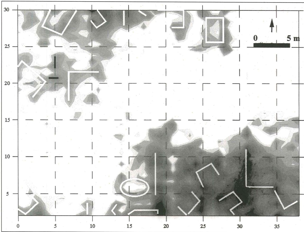
8. EMI data acquired at the Wadi Fidan 4 (WFD 4) site rendered as gray levels. The buried stone walls appear as relative lows and are rendered in black and shades of gray. The superimposed white lines are the interpreted location of walls. All dimensions are in meters.
