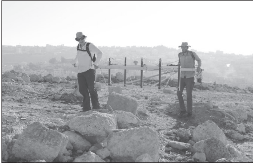
1. The MAG-DRIVE geomagnetic system at work.
