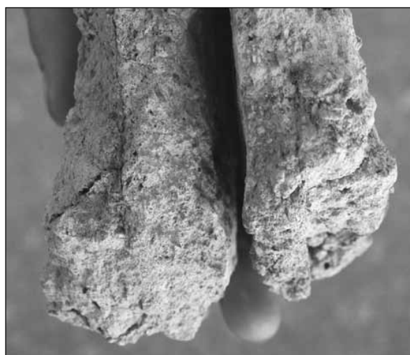
24. Mortar fragments from hypocaust room in ST 20 (Schmid).
