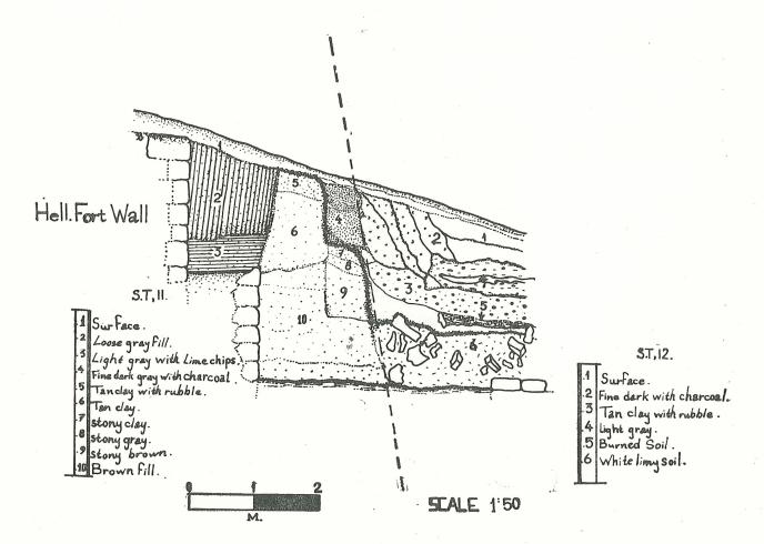
Fig. 1, section of squares 11 (left) and 12 (right).
