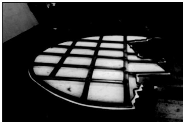
19. A metal bridge was designed to hold the fibreglass, which was attached with screws.
