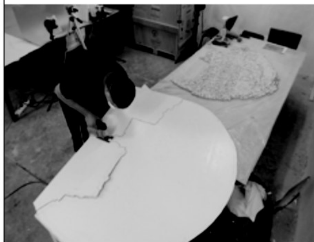
17, 18. A fibreglass board of appropriate size and thickness was designed and then cut to size.
