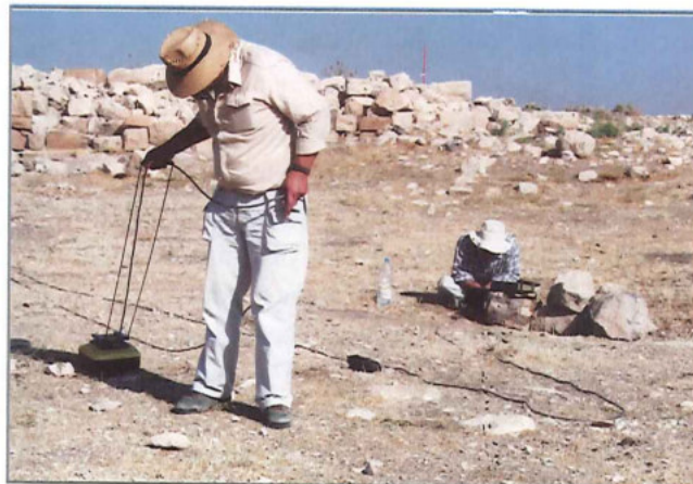
The use of ground penetrating radar greatly enhanced the project's ability to identify sub-surface architectural features.
